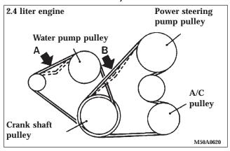
Check the tension of the drive belt. The deflection must be within specifications, when depressed at a point midway between the pulleys as shown in the illustrations with a force of about 100 N (22 lb.).
